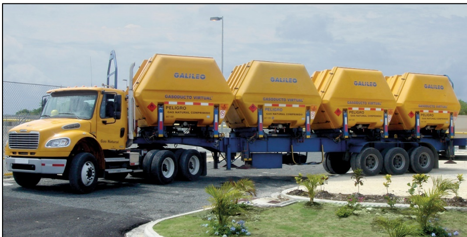
Figure 26 - Example of trailer that would make up virtual pipeline (source: Galileo Technologies).
